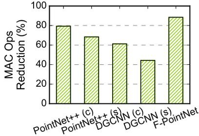
Fig. 9: MAC operation reduction in the MLP by delayed-aggregation. The MAC count reductions come from directly operating on the input points as opposed to aggregated neighbors.
