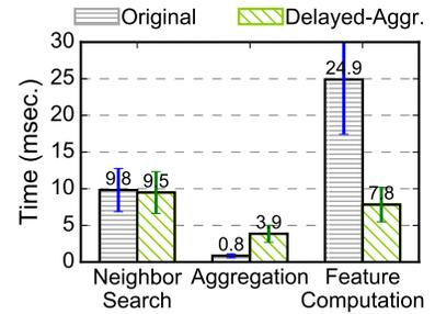
Fig. 11: Time distribution across  $\mathcal{N}$ ,  $\mathcal{A}$ , and  $\mathcal{F}$  in PointNet++ (s) with and without delayed-aggregation. Note that delayed-aggregation would also allow  $\mathcal{N}$  and  $\mathcal{F}$  to be executed in parallel.
