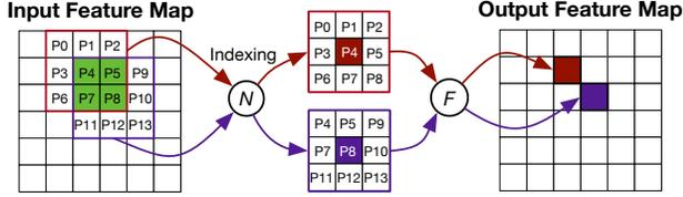
(a) Convolution in conventional CNNs can be thought of as two steps: 1) neighbor search ( $\mathcal{N}$ ) by directly indexing adjacent pixels and 2) feature computation ( $\mathcal{F}$ ) by a dot product.
