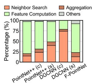
Fig. 5: Time distribution across the three main point cloud operations ( $\mathcal{N}$ ,  $\mathcal{A}$ , and  $\mathcal{F}$ ). The data is averaged on the mobile Pascal GPU on TX2 over 100 executions.
