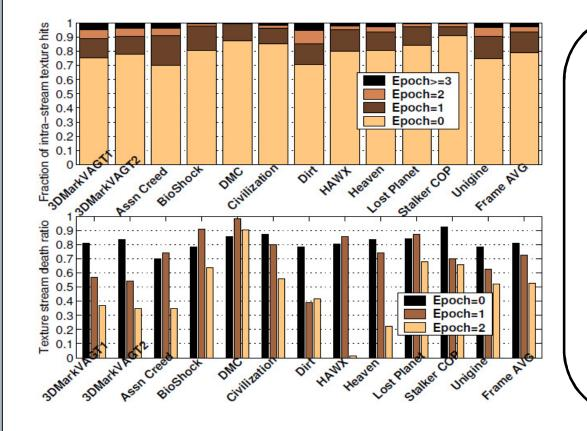
With an optimal LLC policy, most sampler hits come from the  $E_0$  texture partition and almost all hits are covered by the  $E_0$ ,  $E_1$ ,  $E_2$  partitions
