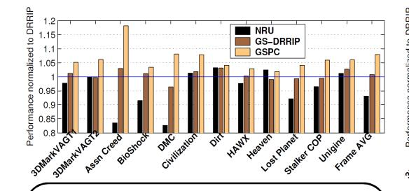
On an 8 MB LLC, the GSPC policy improves frame rate by up to 18.2% and on average 8% compared to DRRIP
