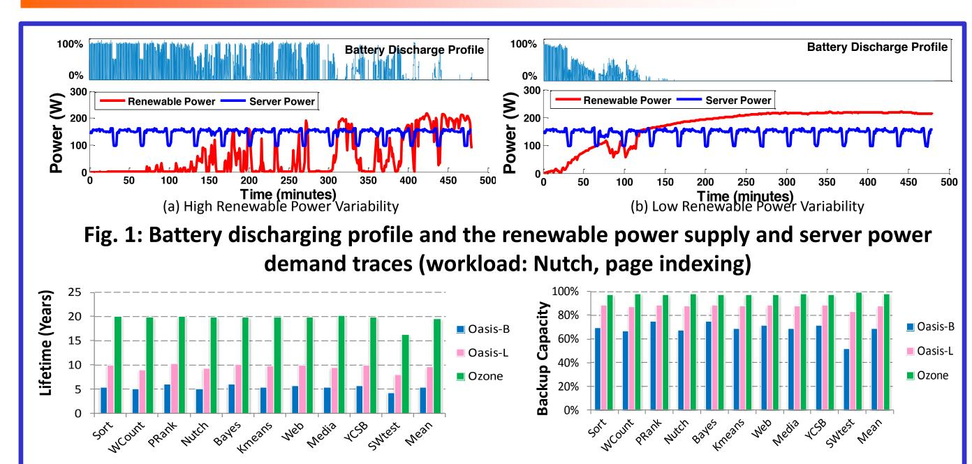
Fig. 2: The estimated battery lifetime
