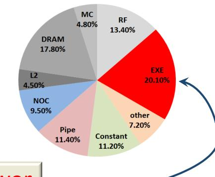
Execution units burn massive leakage and dynamic power Why not power gate the execution units?
