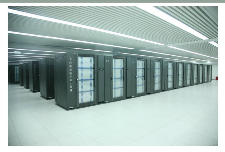
A supercomputer example *TİANHE-1A* Supercomputer (2010) 2,5 petaflops 14336 Intel Xeon processors 7168 NVIDIA Tesla graphics processors
