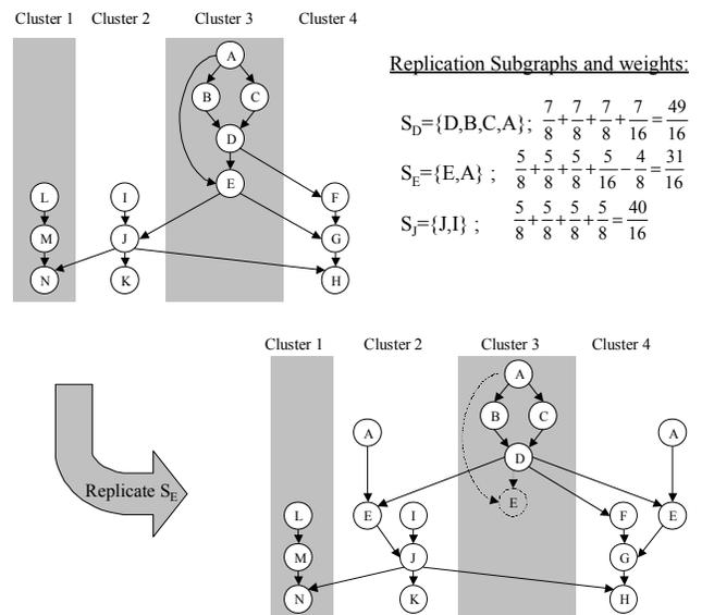
**Figure 3: Example of instruction replication to reduce communications.**
