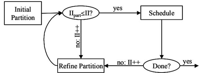
Figure 2: The High level structure of the scheduler.
